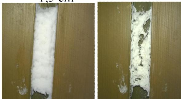
*Figure: Enzymatically fibrillated cellulose + grinded pulp (1:1) + additives. Wet and dry foam in the window slit. Dry content of the water based paste was 13% (w/w). Air content of wet foam 30 %.*
