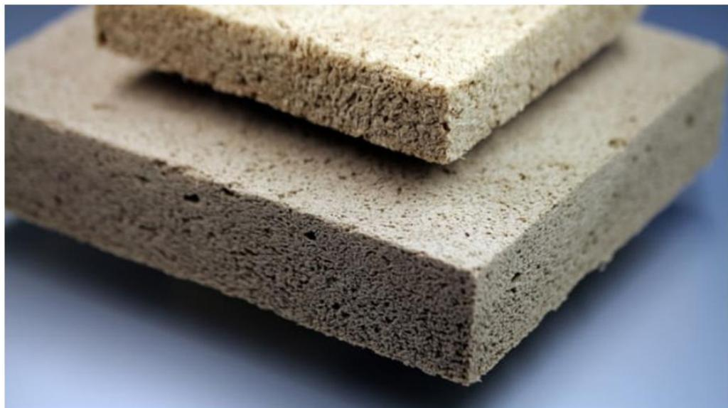
Samples of Fraunhofer's wood foam insulation
