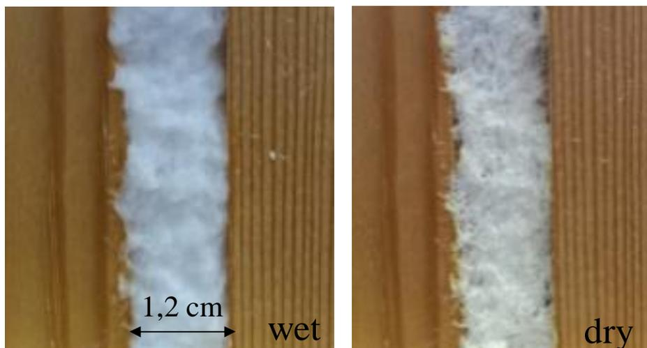
*Figure: Refined pulp (SR 89) based wet and dry foam in the test window slit.*
