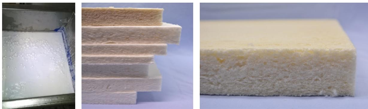
Figure 1. From left: foam forming mould full of wet fibre foam, semi-rigid foam formed thermal insulation panels made of various papermaking pulps, largening of the structure of a foam-formed materials made of 50% softwood kraft and 50% TMP pulp.
