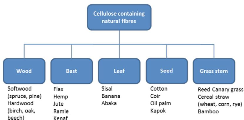
Figure 1. Different sources of natural lignocellulosic fibres.
